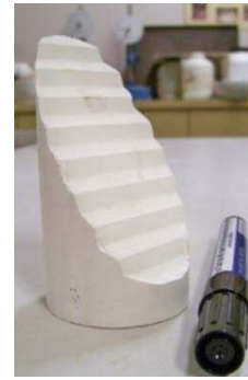
Fig. 1 Simulated joint surface profile of the idealised saw toothed joint
