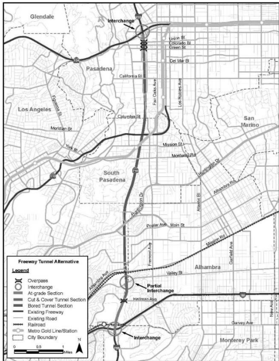
Fig. 1 Freeway Tunnel Alternative Plan
