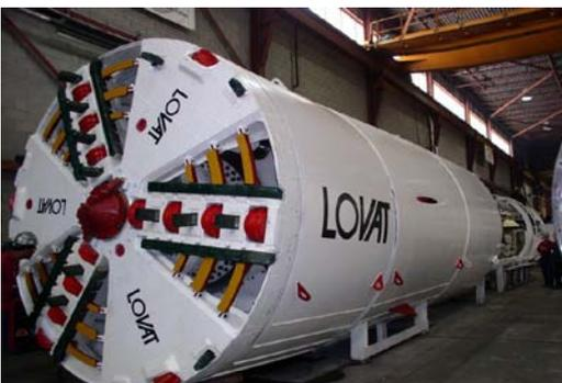
Fig. 4 Pressurized-Face TBM Equipped with Cutterhead for Rock and Soil
