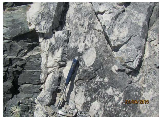
Fig. 1 An example of source rock variability—Partially melted limestone xenoliths embedded within andesitic intrusions resulting difficulties in crushing & screening.
