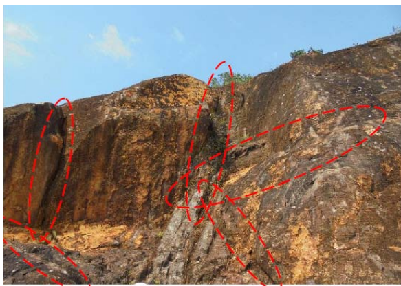
Fig. 4 Joint sets in the bedrock exposed at the top of the slope
