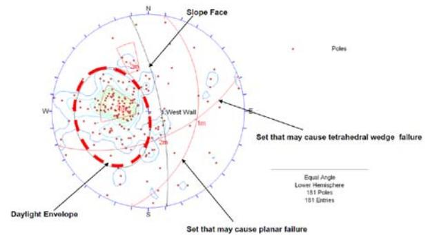
Fig 3. Stereonet of a slope face
