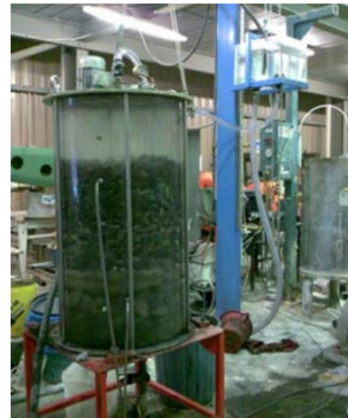
Fig. 3 Large scale permeability test apparatus.
