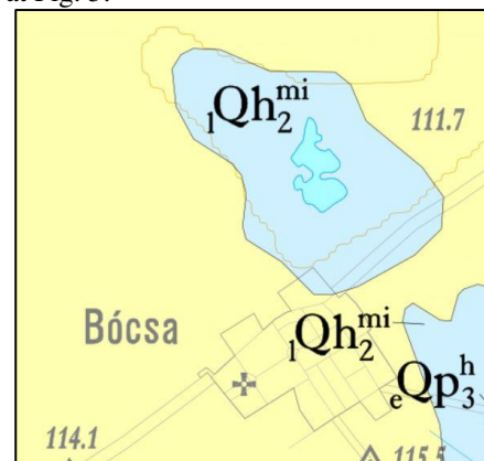
Figure 5. Map of the site. The yellow areas representing the wind-blown sand, while the blue ( 1Qh_2^{mi} ) area is the mud/silt formation
