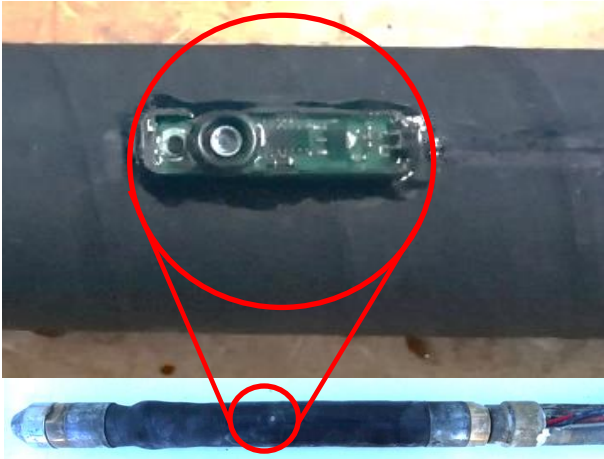
Figure 15. Pore pressure transducer attached to the flexible membrane cover
