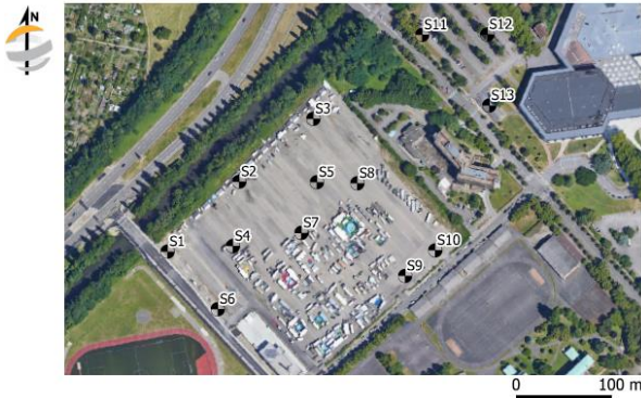
Figure 4. Map layout of the boreholes where pressuremeter tests were carried out.
