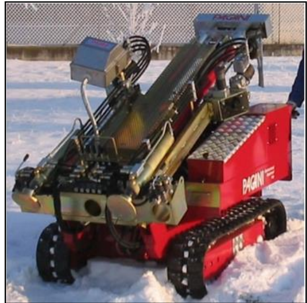
Figure 2. TG63-150 penetrometer. (Source:Pagani)
