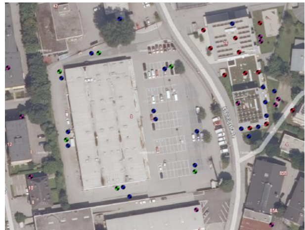
Figure 2. QGIS – extract of the data base: Overview of CPT (red), CPTu (blue), seismic tests (green), core drillings (violet)
