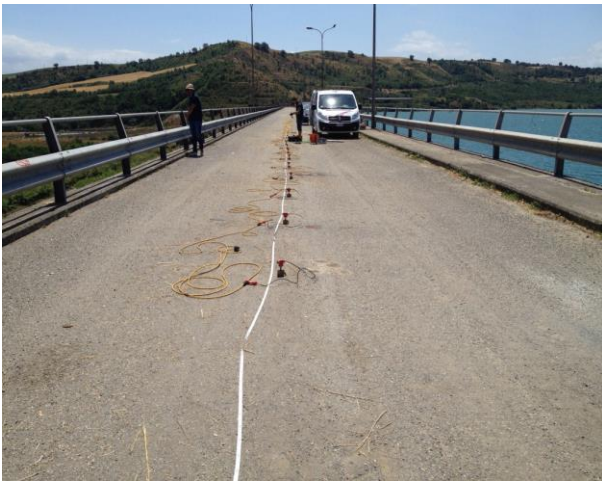
Figure 8. Execution of the MASW test and positions of the receivers.
