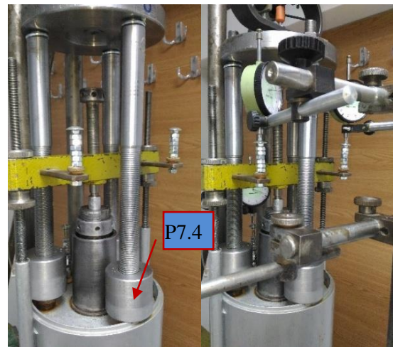
Figure 12. Settlement obstruction using P7.4 (Fig. 6) and disposal of plate pieces in the sample from the sampler, connection of secondary loading collar and putting in place the micro comparators mounted on P13 (Fig. 3)
