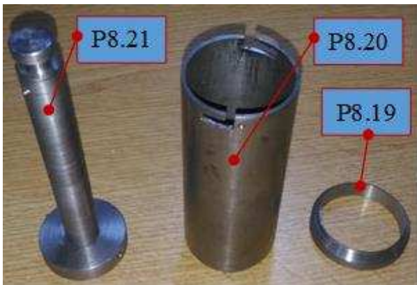
a) Stamp and port stamp (P8.20, P11.3.2) on the pressing ensemble of specimen and guide (P8)
