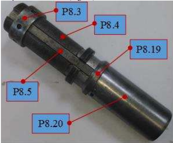
a) Stamp and port stamp (P8.20, P11.3.2) on the pressing ensemble of specimen and guide (P8)
