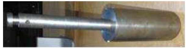
c) Stamp P20 ( \phi 30 mm; h=60 mm) with piece P21 for extraction from sample using P8.1 and P9 from the collar P10, Fig. 5
