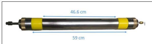
Figure 2. Monocell probe with vulcolan rings
