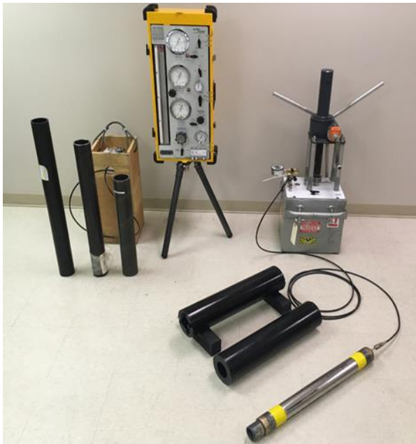
Figure 1. Equipment used: Tricell and Monocell PMT, N-size probe, steel calibration tube, and polyurethane and ABS TST
