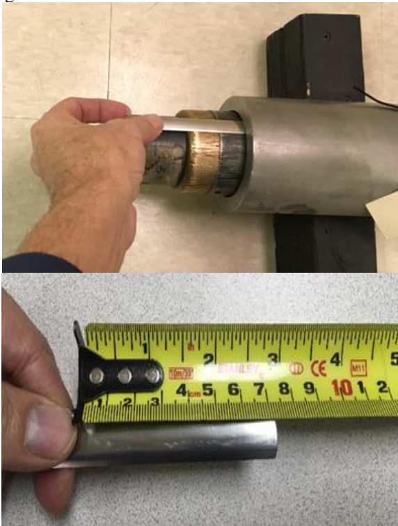
Figure 5. Measuring CL with a steel strip
