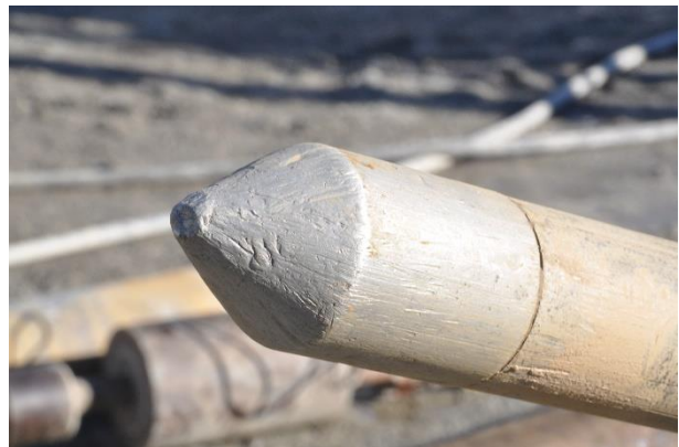
Figure 1. Closed conical tip of an SPT sounding damaged from driving in gravelly deposits.
