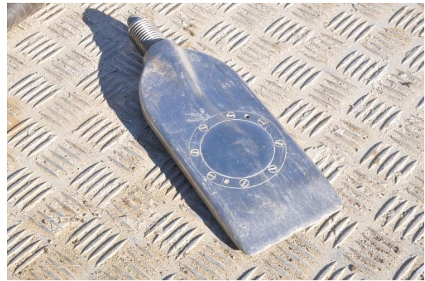
Figure 8. DMT Blade used in fine grained soils with some gravel showing some scratching that may damage the membrane.
