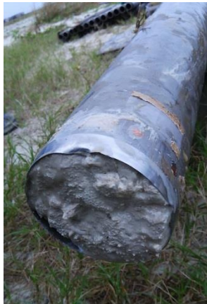
Figure 1. Damage of sharp-edge of a fixed-piston type thin wall sampler
