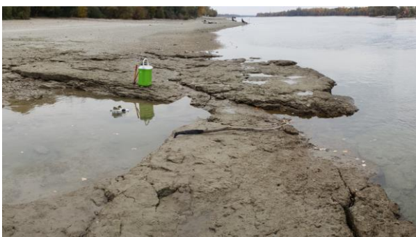
Figure 8. Sample 4, hard to very hard tuffic sandstone layers outcropping at the river bottom nearby Dunakeszi.
