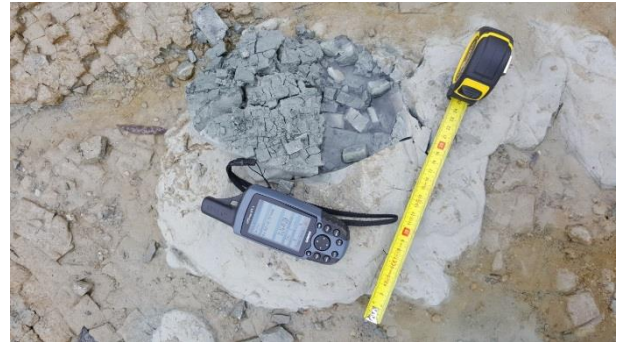
Figure 9. Sample 1, strongly fractured, relatively soft Oligocene clay layer outcropping along the shoreline at Dunakeszi.
