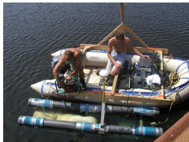
Figure 2. Combined high-resolution seismic and underwater GPR survey performed from a small inflatable boat. Seismic system is towed on the starboard side of the boat, the underwater GPR antenna is mounted on the frame on the port side of the boat.
