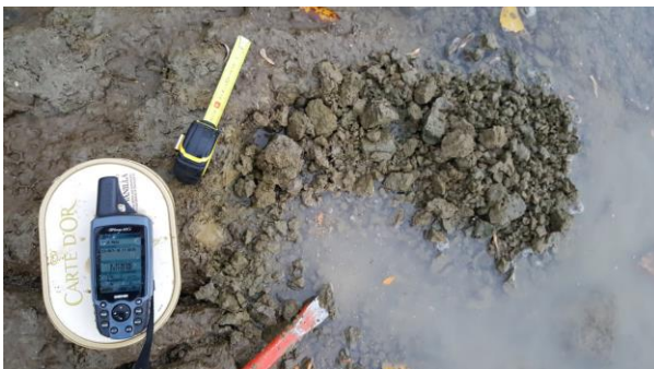
Figure 7. Sample 8, unconsolidated Oligocene Sandstone bed right below the hard tuffic sandstone layer shown in Figure 6.
