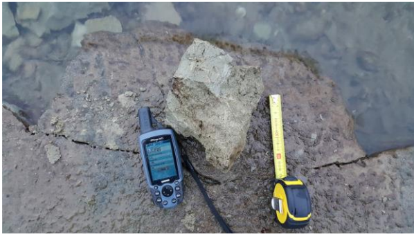
Figure 6. Sample 9, very hard tuffic sandstone layer outcropping at the river bottom nearby Göd.
