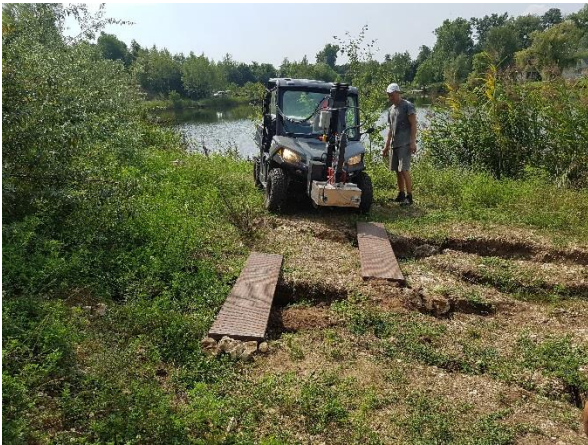
Figure 5. Lightning™ seismic source in the survey area crossing a surface crack zone
