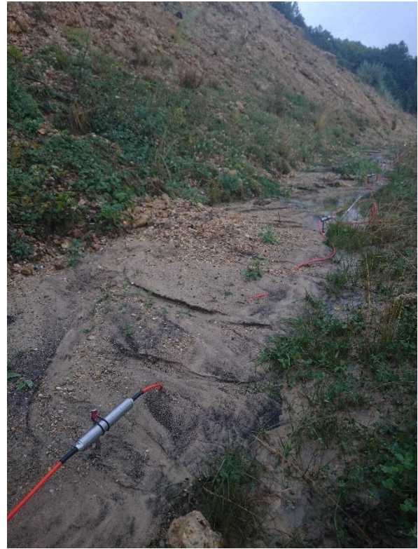
Figure 4. Electrical tomography profile measured in strike direction on the slope. Please note the amount of eroded sediment caused by a heavy rainfall during the measurement.
