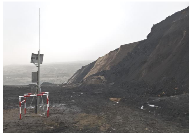
Figure 15. The on-line monitoring station in Belchatow mine.
