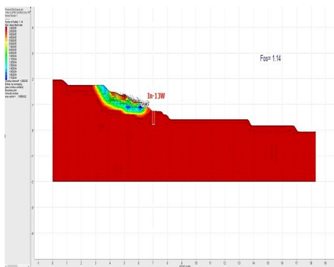
Figure 23. Slope stability analysis 20WE, SSR method, Fos = 1.14.
