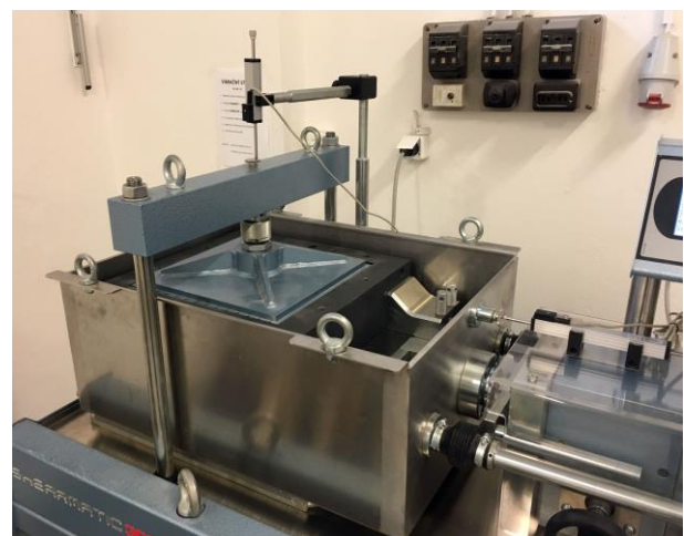
Figure 1. Large-size direct shear test apparatus
