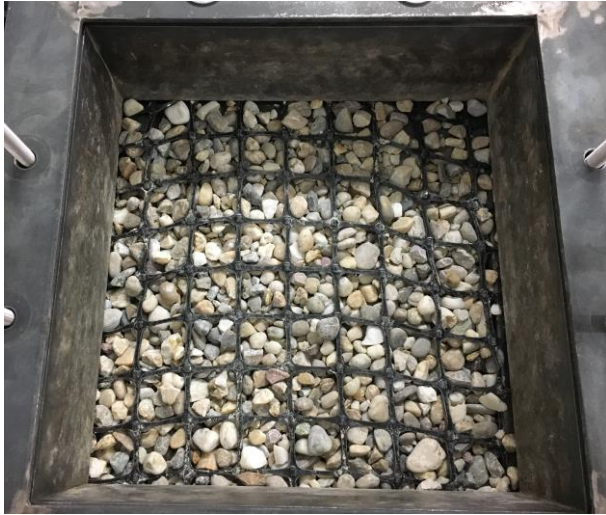
Figure 2. Fixing the geogrid to the upper part of the shear box
