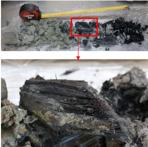
Figure 6. CPT sample pushed at the level of the mine roof at CPT2a: 500mm of recovered material with EW siltstone to the left and coal fragments to the right (top); enlargement of hardwood timber fragment push-cored by the sampling tube (bottom).
