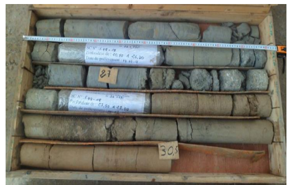
Figure 10. Compact marl interspersed with sandstone
