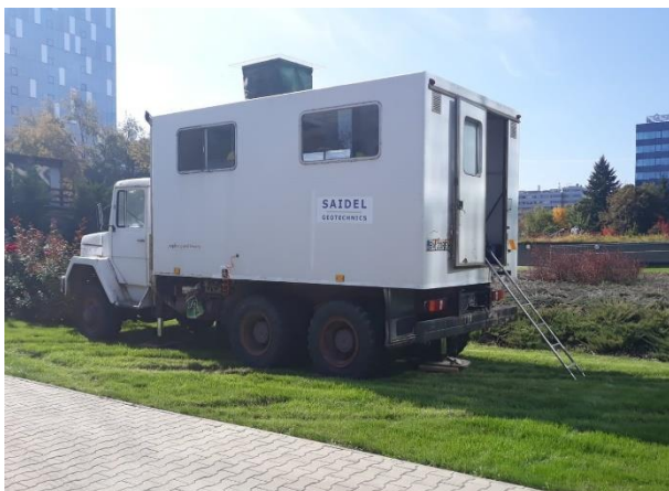
Figure 1. CPT Truck used to push the CPT cone and the DMT blade into the ground
