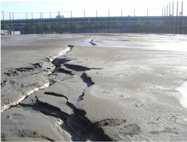
Figure 4. Liquefaction damage in Urayasu City during the 2011 Tohoku earthquake, Japan.
