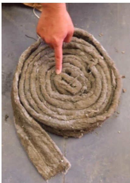
Figure 5. Detected plastic drain that made jet grouting difficult and costly.
