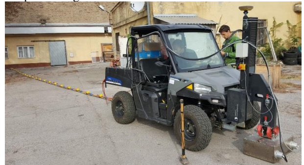
Figure 1. The land streamer system with electromagnetic S-wave vibrator and P-wave hammer in urban area.
