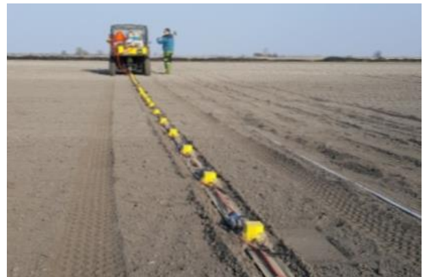
Figure 2. The land streamer system with electromagnetic S-wave vibrator and P-wave hammer on agricultural test site.
