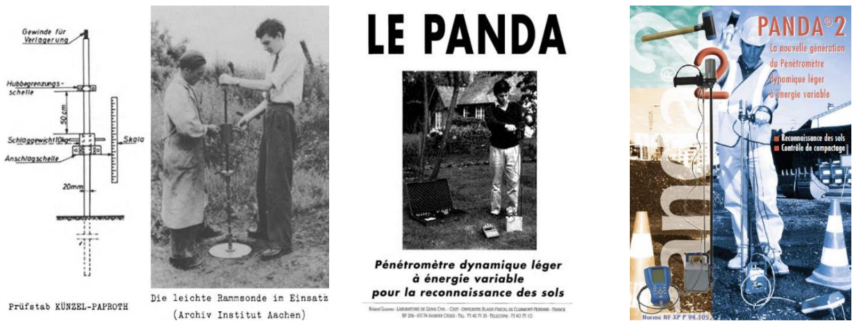
Figure 1. (a) Prüfstab Künzel-Paproth" (Menzenbach, 1959) (b) P.A.N.D.A.® lightweight dynamic variable energy penetrometer: first generation (Gourvès R. , 1991) and (c) P.A.N.D.A. 2®: second generation.
