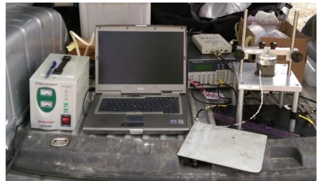
Figure 8. Test set up for shear wave velocity measurements on unconfined samples in the field (Photo Priscilla Paniagua)
