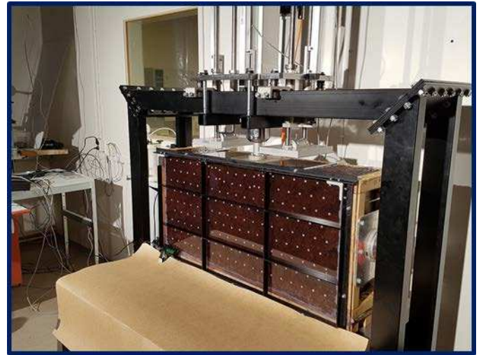
Figure 14. Test set up for 1g laboratory model tests.
