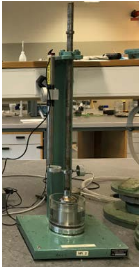
Figure 7. Set-up for the Janbu torvometer apparatus.
