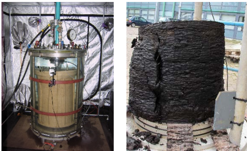
Figure 5. Large triaxial tests left: test set-up right: sample after testing. From: [7]
