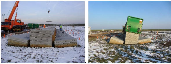
Figure 1. Test number 6 at the Uitdam test site. Left; Application of extra load to the pre-loading. Right; test set up at failure
