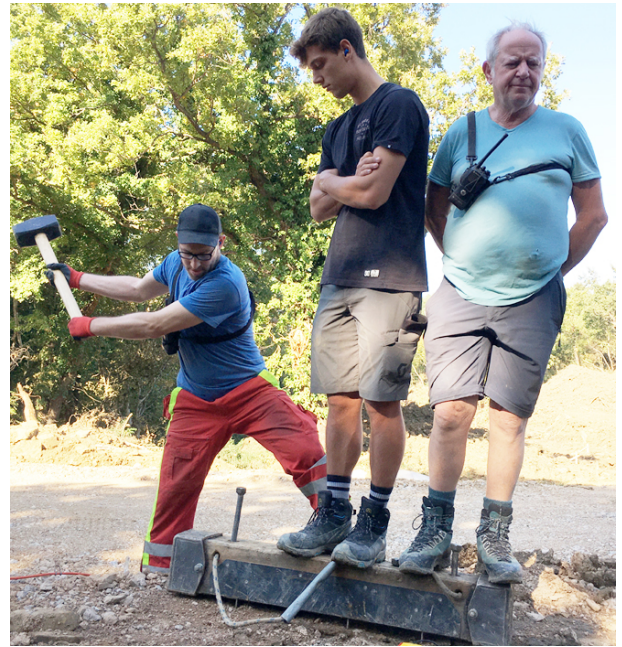
Figure 2. Shear wave source A square-shaped timber coupled to the ground and a 8 Kg sledgehammer impacts the end-grained side;
