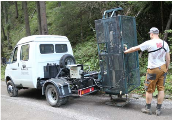
Figure 10. : Accelerated dropweight (4x4 light-weight truck mounted Bison EWG Mark III®) as seismic source for a combined P-wave / MASW survey deployed in an Alpine karstified operational theatre
