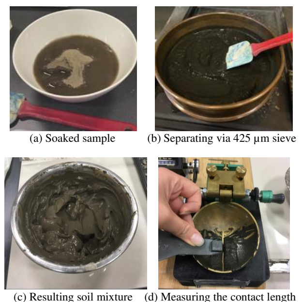
Figure 14. Determination of liquid limit
