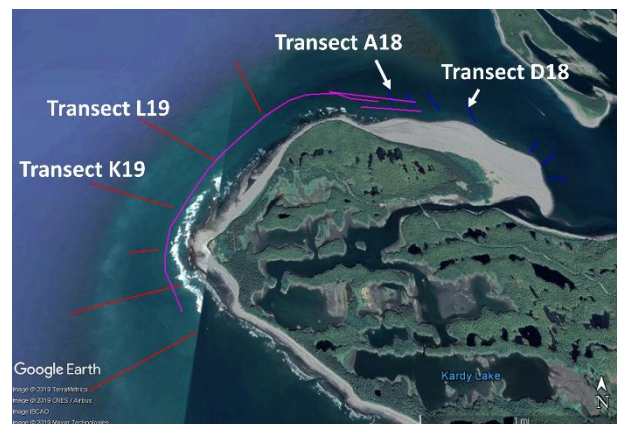
Figure 5. Google Earth (2019) image with measured transect lines: cross-shore transects measured in 2018 in blue, cross-shore transects measured in 2019 in red, and longshore transects in magenta. Transects of relevance to this article are labeled [31].
