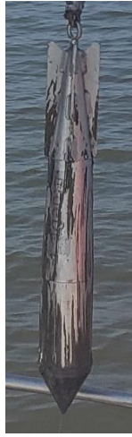
Figure 4. Photo of PFFP BlueDrop after deployment in muddy sediments.
