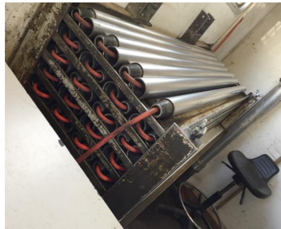
Figure 1. A schematic diagram of a long cable passing through the probe rods
