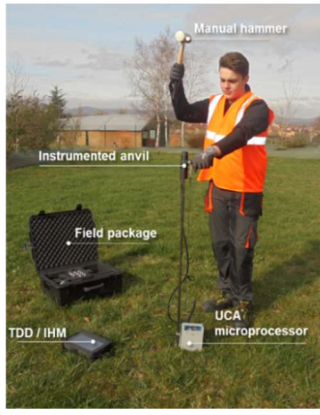
Figure 3. (a) Dynamic penetrometer Panda 3 ® apparatus, (b) Example of Panda 3 ® raw data (force, acceleration and displacement signals) recorded for one single blow [17] and (c) Experimental shock polar curve obtained for different materials (steel rods, concrete, wood and sand). [17]
