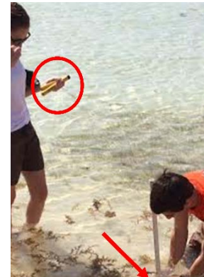
Figure 11. Deployment of RBR SoloD pressure transducers during an undergraduate research field experiment in a sandy nearshore zone in the Punta Cana, Dominican Republic.
