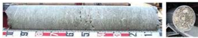
Sample core of fragmented shell in dense sand (GP-D: 200 mm).
