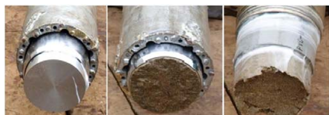
(a) Photo of free piston (b) After sampling (c) Bit and shoe removed
