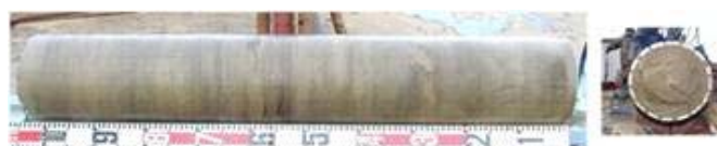
Dense sand sample core (GP-D: 200 mm).
