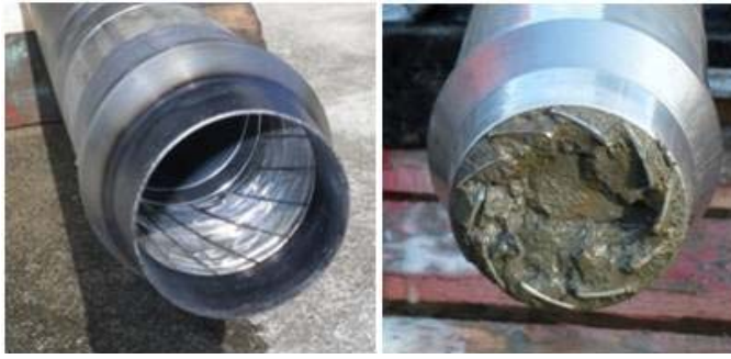
(a) Shoe and core catcher with piston removed. (b) Activated core catcher with sample inside.
