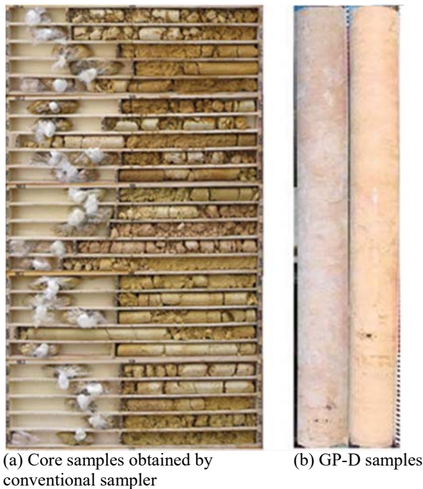
Figure 31. Photos of Ryukyu Limestone core samples obtained by conventional sampling and GP-D sampler (Arikawa et al. 2008)
