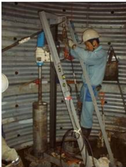
Figure 15. Photo of GP-R sampling inside the deep well at Ohkubo Block (Supplied by Mt. Fuji Sabo Office).
