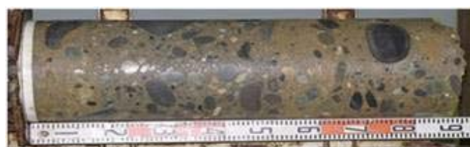
Sample core of gravels suspended in a matrix of dense sand (GP-R: 300 mm).
