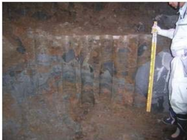
Figure 17. A photo of suspected slip surface at Hachigasawa Block at a depth of 42 m (Supplied by Mt. Fuji Sabo Office).
