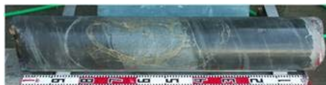
Sample core of mudstone (GP-R: 200 mm).
