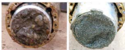
Figure 40. Soil profile at Padma site, and samples obtained at 58 m (left) and at 84 m (right).
