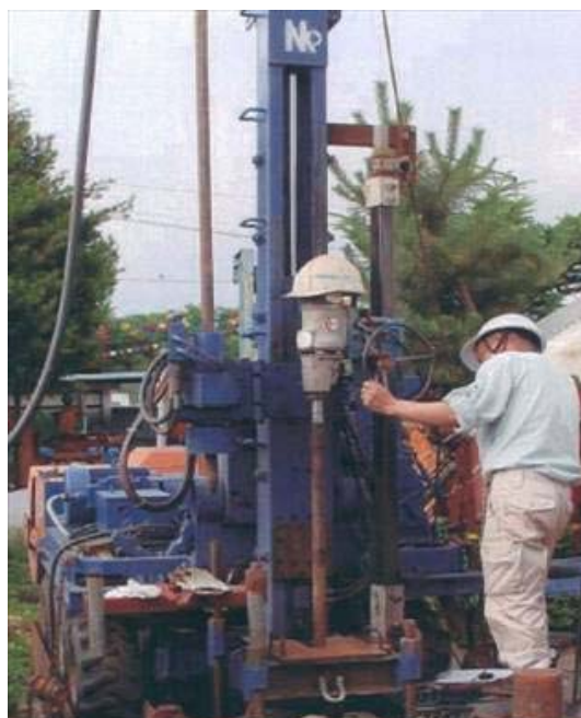
(c) Photo of GP-D sampling using an electric motor.
