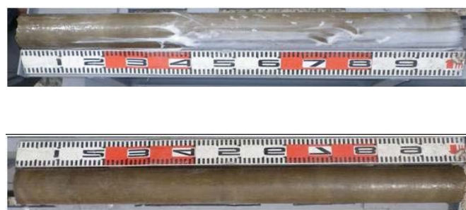
Figure 36. Photos of GP-Tr sample extruded out of the liner tube (above) and polymer solution wiped off (below).
