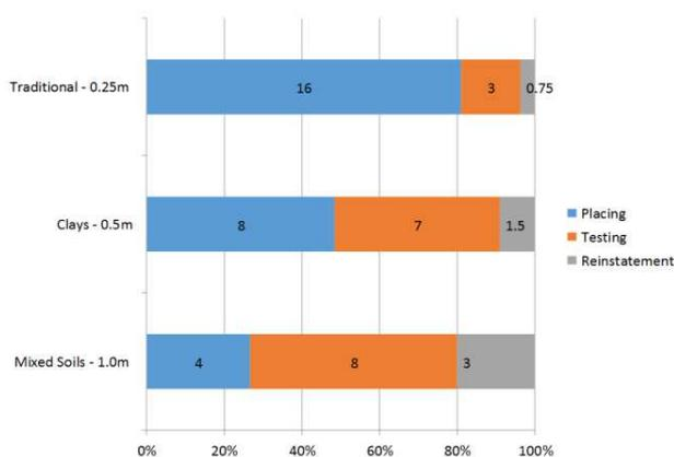
Figure 2. Typical Time (hrs) of various compaction activities for 4,000m<sup>3</sup> with 8 sand replacement tests (Look, 2012).
