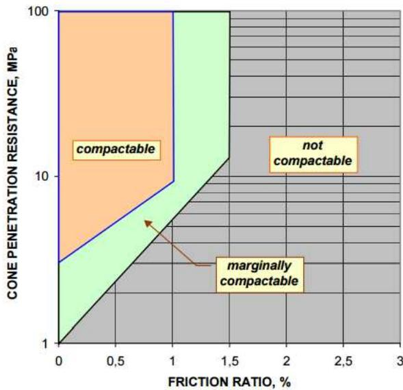
Figure 5. Soil classification for deep compaction based on CPT (Massarsch, 1998).
