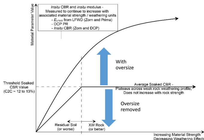
Figure 9. Comparisons between in-situ modulus and soaked CBR tests.
