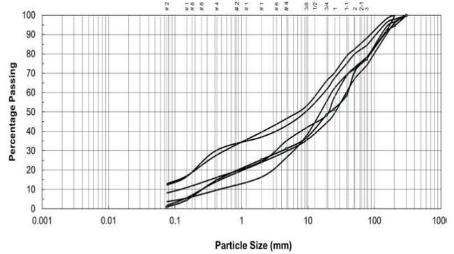
Figure 14. Particle size distribution curves rock-fill materials
