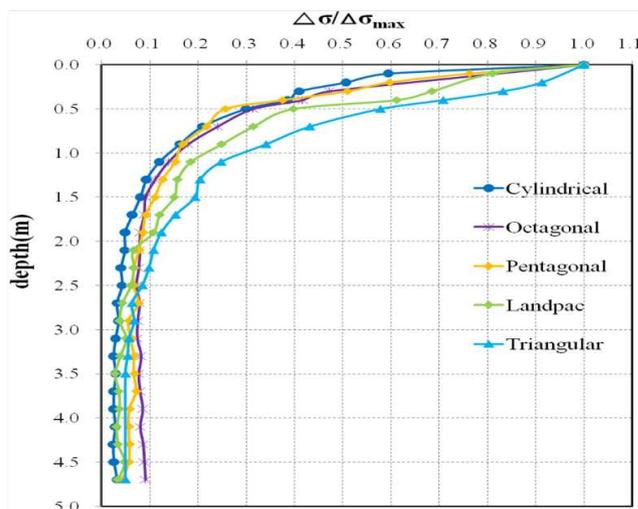
Figure 3. Depth of Influence for various shape rollers based on finite element analysis (Briaud & Saez, 2012).
