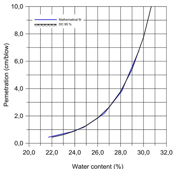
Figure 8. Compaction control as a function of the PI and moisture content, considering a degree of compaction greater than 95%.
