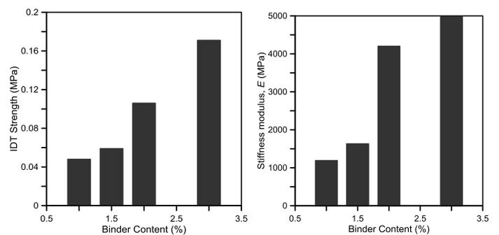
Figure 6. Variation of IDT strength and stiffness modulus with binder content.
