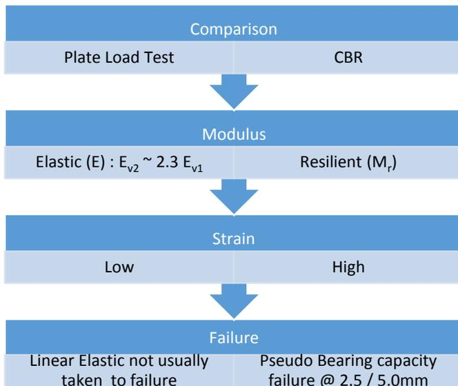
Figure 10. Comparisons between PLT and CBR tests.
