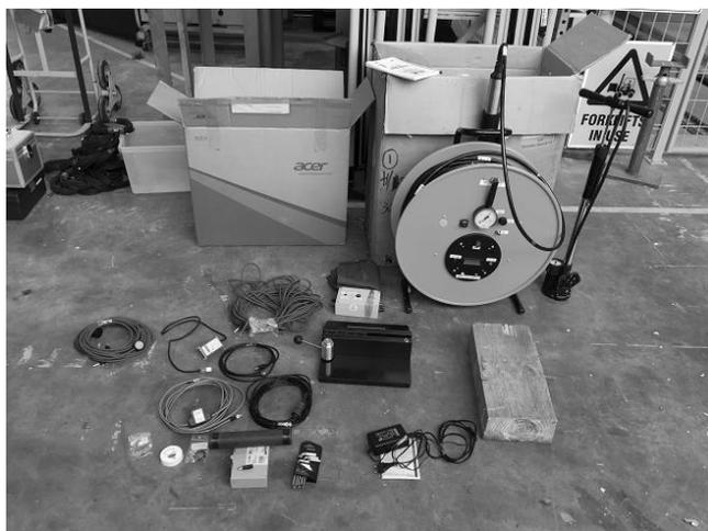
Figure 6. Geotomographie™ borehole geophone and other equipment used for P-S logging in DCPT-7.
