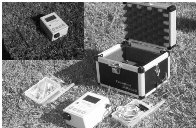
Figure 1. Tromino™ velocimeter used for HVSR technique.
