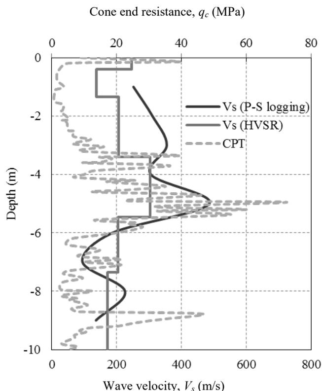
Figure 7. Normalised HVSR  $V_s$  versus normalised CPT  $q_c$  versus normalised P-S logging  $V_s$ .
