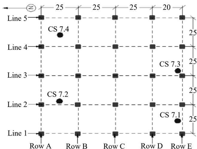
Figure 2. Observation stations of the compacted area (dimensions are in metres).
