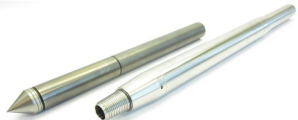
Figure 4. Magneto module with 10 cm 2 Icone.
