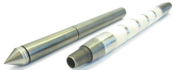
Figure 3. Conductivity module with 10 cm 2 Icone.
