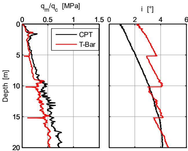
Figure 3 T-bar inclination changes during cyclic test stages compared to a cone penetration test; cyclic test stages are evident from low-value spikes in  $q_m$  profile.
