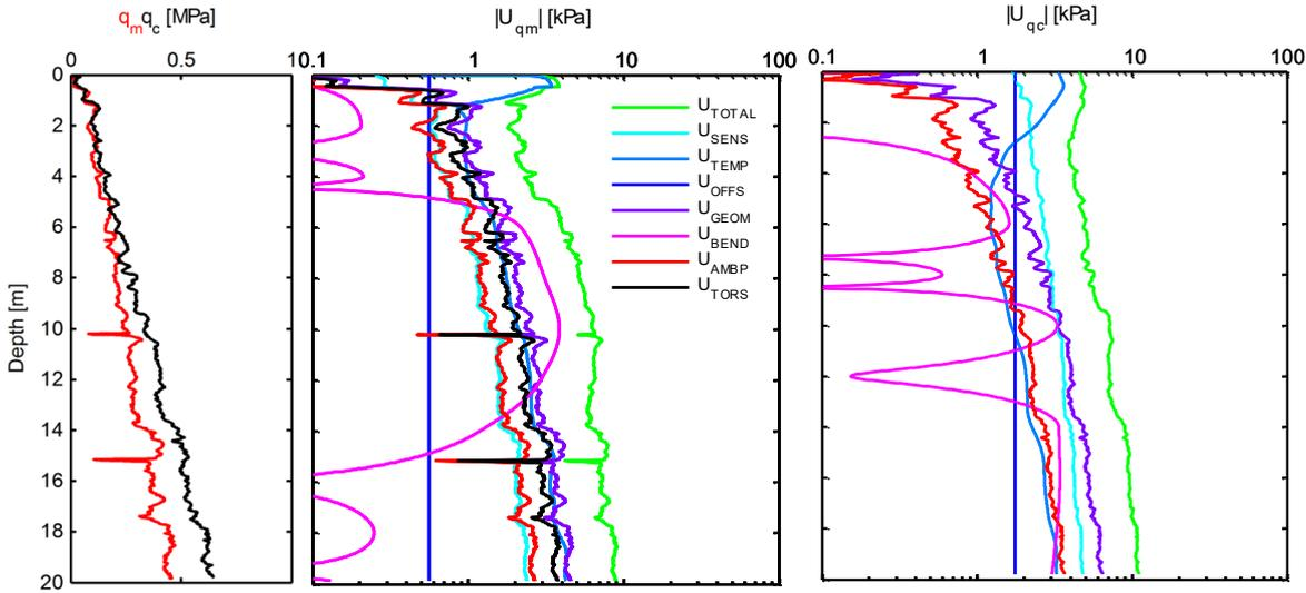
Figure 2 Examples of uncertainty estimates for high-quality TBT and CPT systems and practices, non-drilling deployment and water depth of 1500 m.
