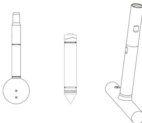
Figure 1 Fugro T-bar, cone and ball penetrometers.
