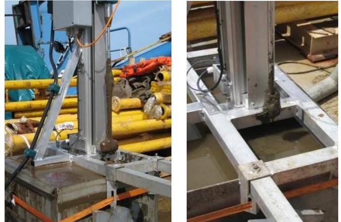
Figure 4 Soil adhering to mini T-bar penetrometer after retraction from offshore box core sample.
