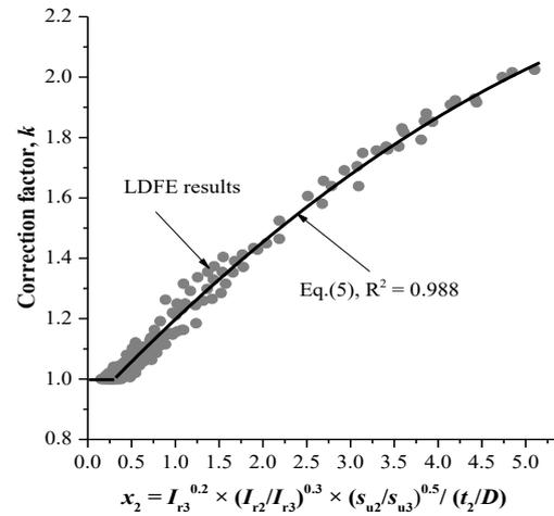
Figure 6. Design chart for correction factor  $k$  accounting for effect of soil stiffness
