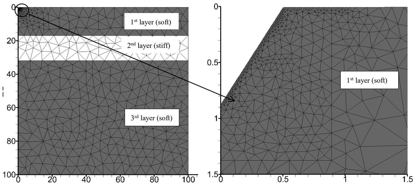
Figure 2. Initial mesh for cone penetration in soft-stiff-soft clay (axes normalized by cone diameter  $D$ )
