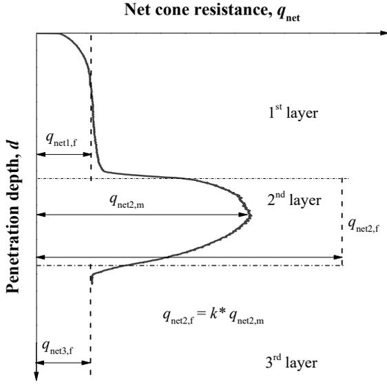
Figure 4. Typical penetration resistance profile in soft-stiff-soft clay and thin-layer correction factor  $k$  for 2<sup>nd</sup> layer
