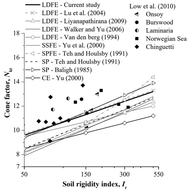
Figure 3. Effect of soil rigidity index on piezocone deep bearing capacity factor  $N_{kt}$
