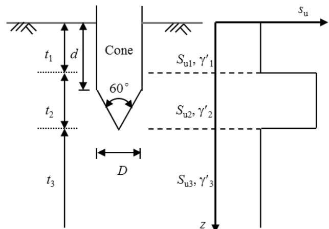
Figure 1. Schematic diagram of cone penetration in soft-stiff-soft clay
