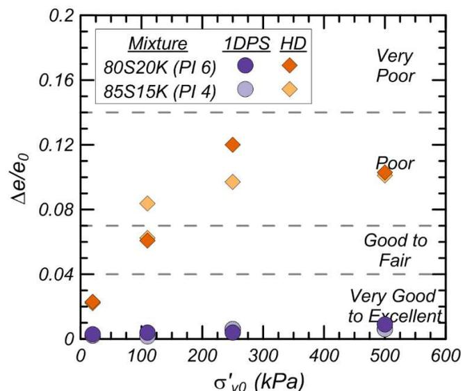
Figure 6.  $\Delta e/e_0$  sample quality rating for 1DPS and HD specimens for 4 different simulated in-situ stress levels and two different mixtures: 80S20K (PI 7) and 85S15K (PI 4).
