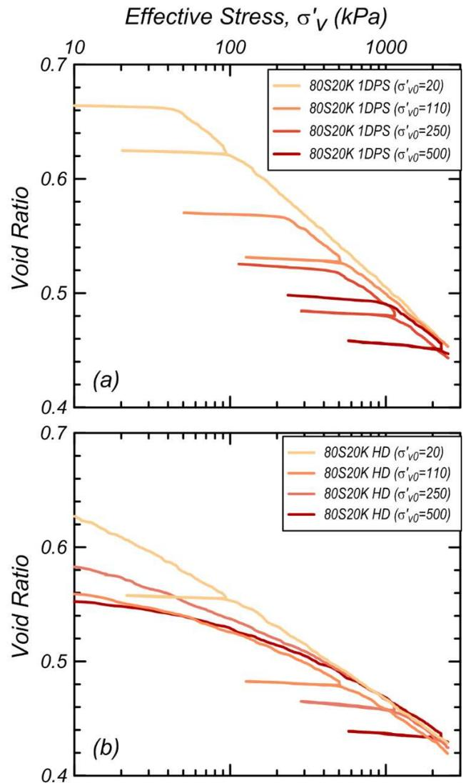
Figure 5. Plots of void ratio versus effective stress for (a) 1DPS and (b) HD loading of 80S20K for 4 simulated in-situ stress levels.
