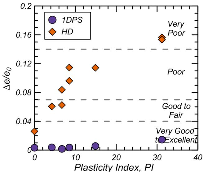
Figure 2. Results from a study using synthetic intermediate soil mixtures indicate a strong trend of increasing sample quality with decreasing PI for heavily disturbed mixtures.
