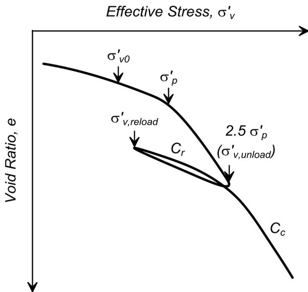
Figure 4. Conceptual loading path for phase 3 loading.
