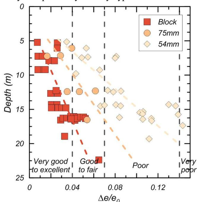
Figure 1 – Sample quality for different sampling methods: Sherbrooke Block, 75mm piston, and 54mm piston samplers. Dashed lines are added to indicate trend with depth (overburden stress) for each sampling method. Note that each sampling method was performed on three different clay soils.
