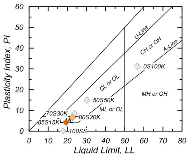
Figure 3. Atterberg limits for the synthetic intermediate soils where colored symbols indicate mixtures used in this study and gray symbols indicate mixtures used in Krage et al. (2015).
