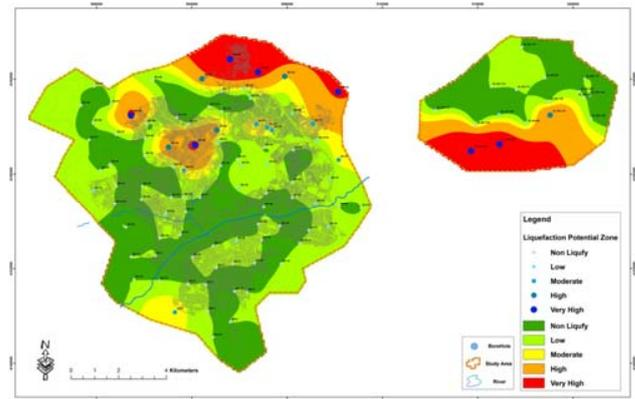
Figure 4. Urmia Liquefaction potential map
