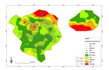
Figure 4.Urmia Liquefaction potential map
