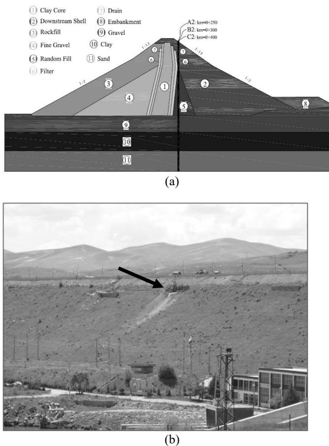
Figure 2. (a) Main section and borehole positions at Mahabad Dam (b) A view from downstream slope of the dam and placement of the drilling equipment near the crest
