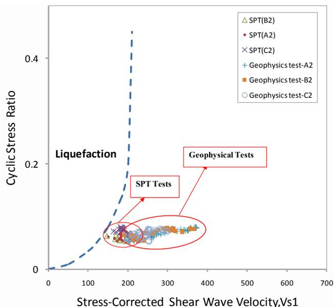
Figure 4. Liquefaction potential assessment at Mahabad Dam body and foundation, cyclic shear stress ratio (CSR) vs. stress-corrected shear wave velocity ( $V_{s1}$ )
