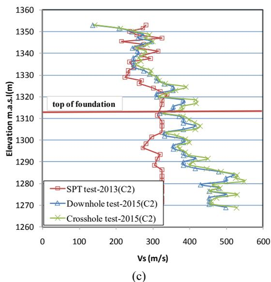
Figure 3. Shear wave velocity profiles for (a) A2, (b) B2, and (c) C2 boreholes obtained by SPT, down-hole and cross-hole tests
