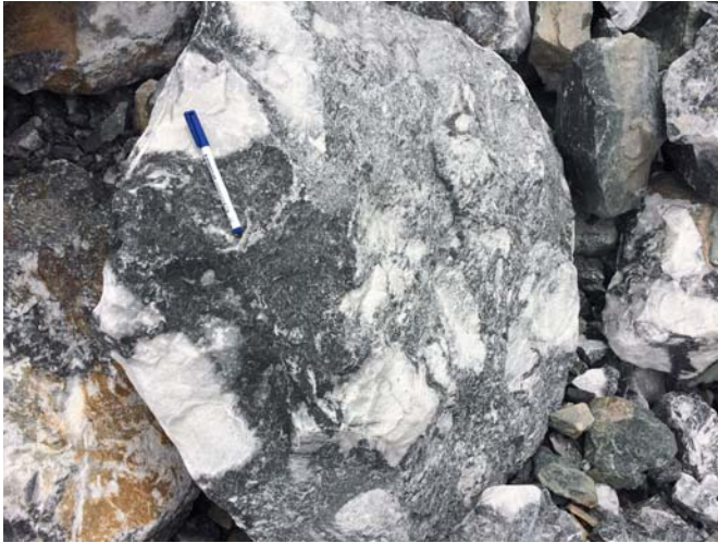
Figure 1. An example of source rock variability - Partially melted/liquefied dolomitic limestone xenoliths (white patches) embedded within andesitic intrusions resulting processing and sorting difficulties.
