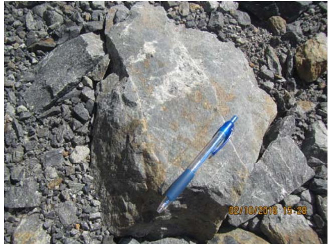
Figure 4. An example of iron sulphide bearing regional metamorphic source rock showing scattered pods and vugs of gold-
