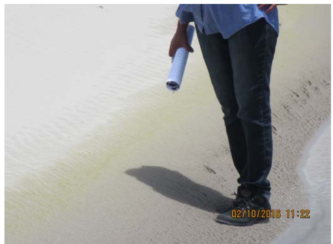
Figure 6. Formation of jarosite ( \text{KFe}_3(\text{OH})_6(\text{SO}_4)_2 ) with yellow band along the moisture front due to aerial oxidation of pyrite ( \text{FeS}_2 ) in a stockpile of processed fine natural sand aggregate sourced from tidal sand deposit. This reveals the pres-
