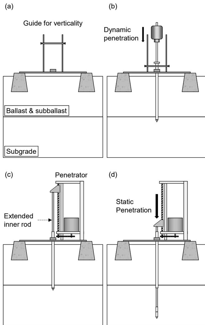
Figure 4. Test procedure of DSCP: (a) installation of a guide for verticality; (b) dynamic penetration of the DSCP; (c) installation of a penetrator; (d) static penetration of the DSCP.
