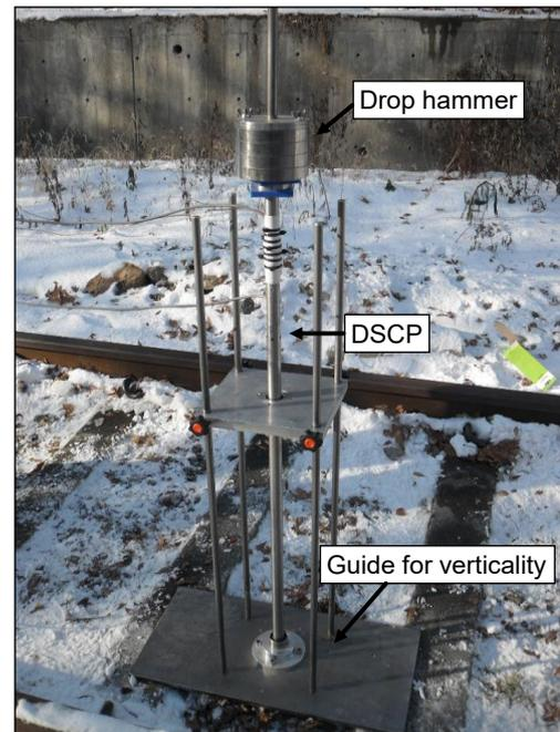
Figure 5. Photographic image of the dynamic penetration of DSCP.
