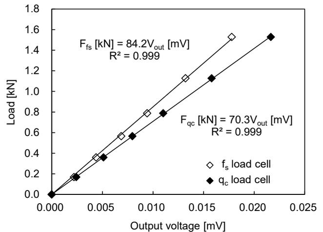
Figure 3. Relationship between the output voltages and the loads acted on the  $q_c$  and  $f_s$  load cells.  $F_{q_c}$  and  $F_{f_s}$  denote the loads acted on the  $q_c$  and  $f_s$  load cells, respectively.
