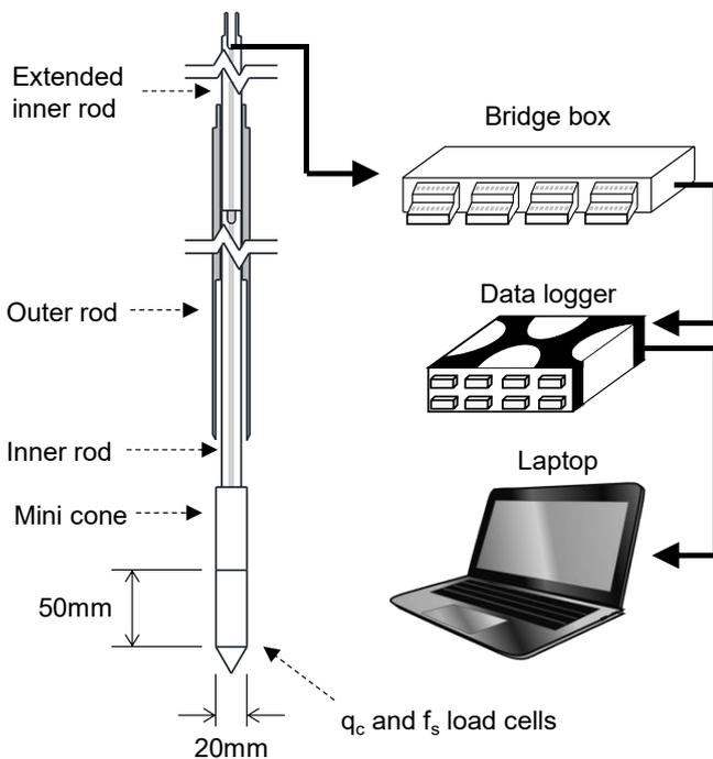
Figure 2. Schematic drawing of DSCP and the measurement system.
