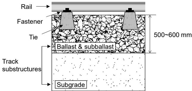
Figure 1. Cross-section of the railroad system.
