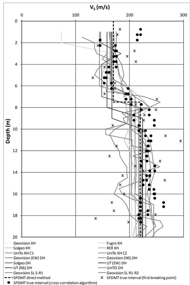
Figure 4. Comparisons between CH, DH suspension logging results of the InterPACIFIC project (grey lines, Garofalo et al. 2016) and SPDMT results (black line and symbols) in terms of  $V_S$  and  $V_P$  values at Mirandola test site.
