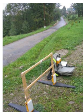
Figure 2. GPR, 100 MHz unshielded antennas, landslide No 21
