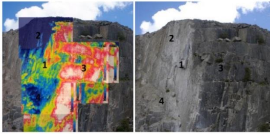
Figure 8. (a) Thermal images draped over point cloud of same position depicted in figures 6 and 10 (b) Raw format digital image of same exposure aids identification of specific features.
