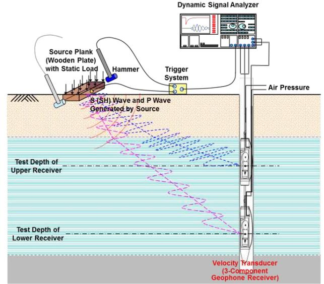
Figure 2. Schematic diagram of an in situ downhole seismic test in a borehole.
