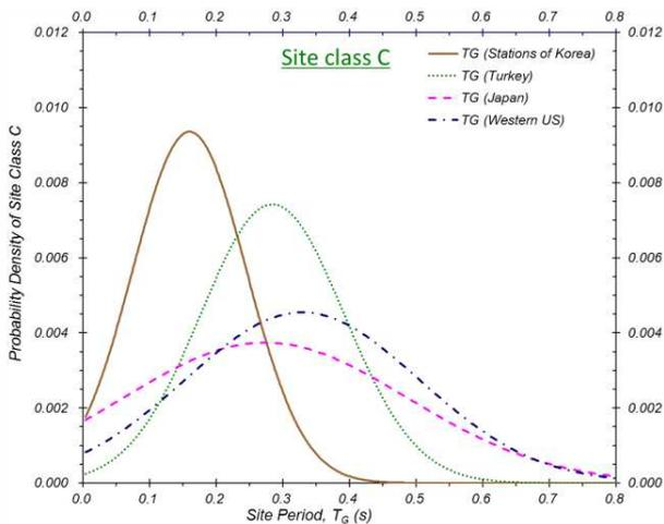
Figure 9. Comparisons of the probability distributions of  $T_G$  for seismic stations of site class C in Korea and strong seismicity regions.
