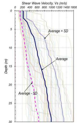
Figure 3. Average  $V_S$  profile to 30 m depth based on the  $V_S$  profiles at the sites in South Korea.
